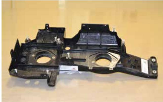
Engine mount of glass-mat-reinforced thermoplastic in combination with thermo-prepreg, which can be manufactured at the IST, thanks to the rapid pressure build-up in the press
