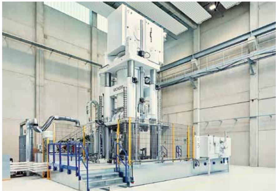
WKP 25000S: The composite press is accessible all round and can be operated from two sides
